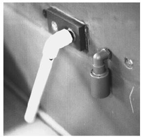
Return line / Right-Angle Etch full float (Inside etcher)
