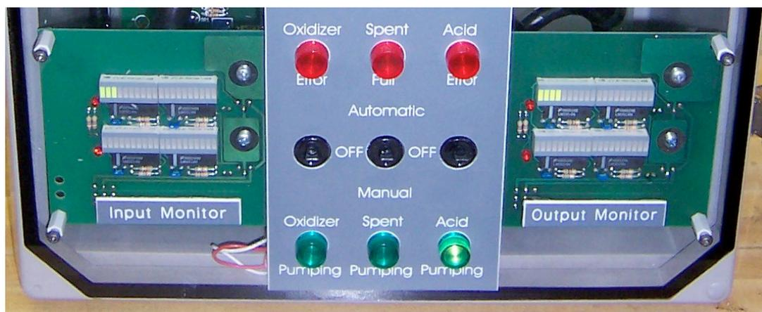
**Front Panel Switches, Input And Output Monitors**
